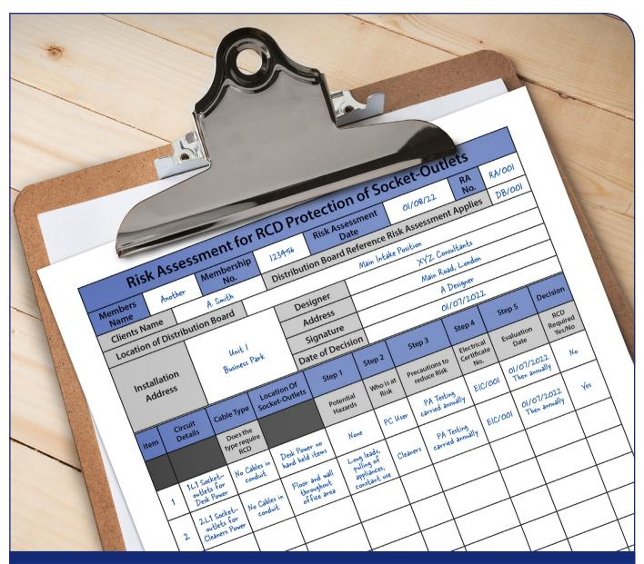
Fig 1: Example of a risk assessment to omit an RCD from a socket-outlet, in accordance with Regulation 411.3.3
